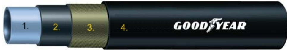
1. Tube – FPM (FKM); 2. Tie – NBR; 3. Reinforcement – PET braid; 4. Cover – CM (CPE)
